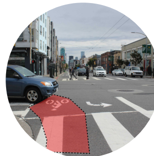
Lack of bicycle infrastructure to support cyclists making right turns onto Howard. Causes cyclists to use pedestrian crosswalk instead of staying in the bike lane.
