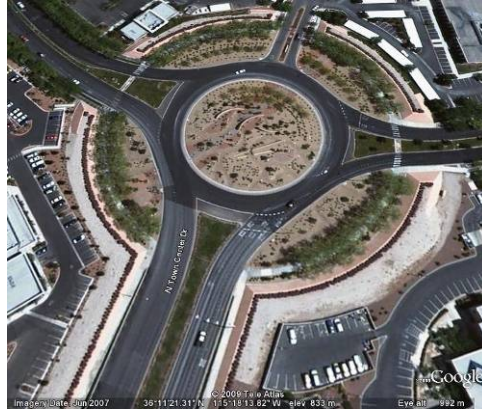
Figure 7: Roundabout with unlimited sight distance
