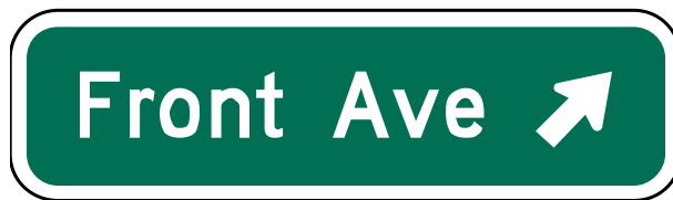
Figure 17: MUTCD Recommended Exit Sign for Roundabouts (FHWA, 2008)
