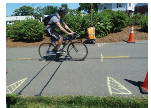
Bicyclist riding over piezoelectric strips.
