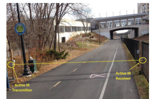
Active infrared counter installation at a test site.
