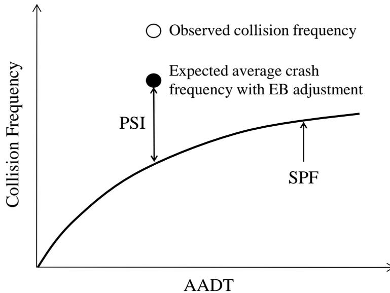
Fig. 4. PSI Estimated for Three Network Screening Methods
