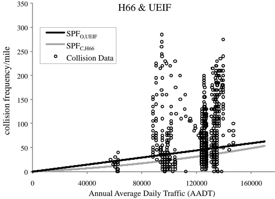
Fig. 3.  $SPF_{O,UEIF}$  and  $SPF_{C,H66}$  for the Corresponding Collision Data
