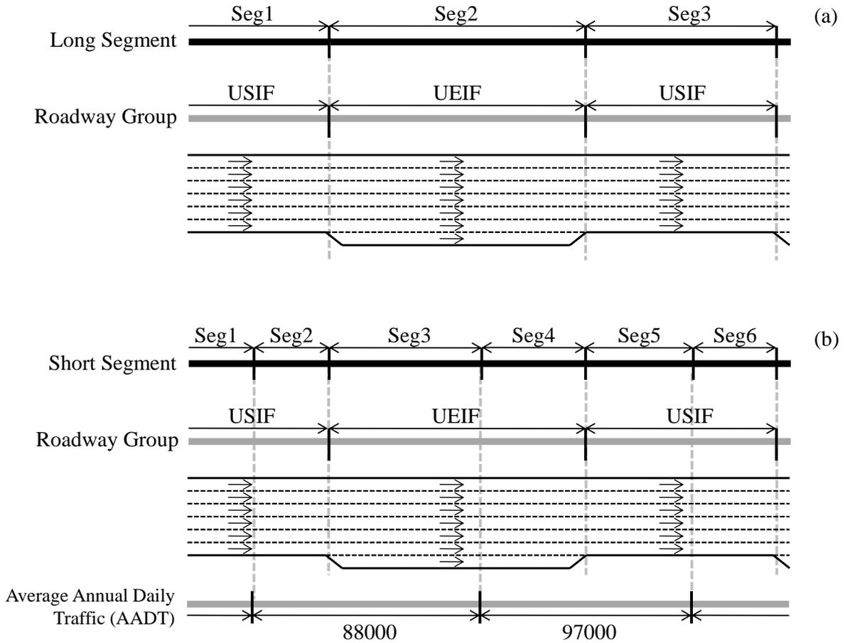
5 Fig. 2. Two Ways to Define Roadway Segment: (a) Long Segment, (b) Short Segment
