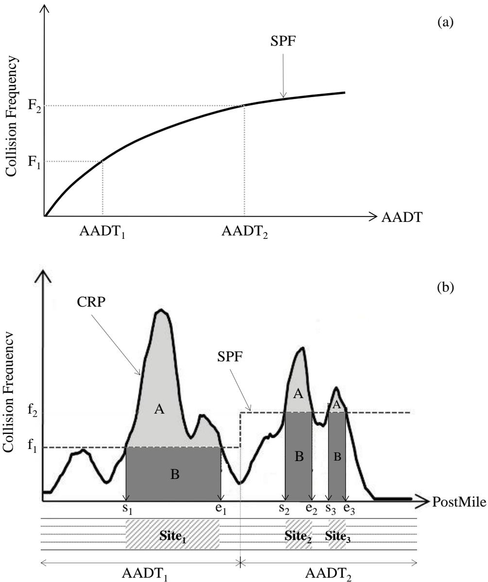
1 Fig. 7. Continuous Risk Profile (CRP) Method: (a) Predicted Collision Frequency, (b) Site
