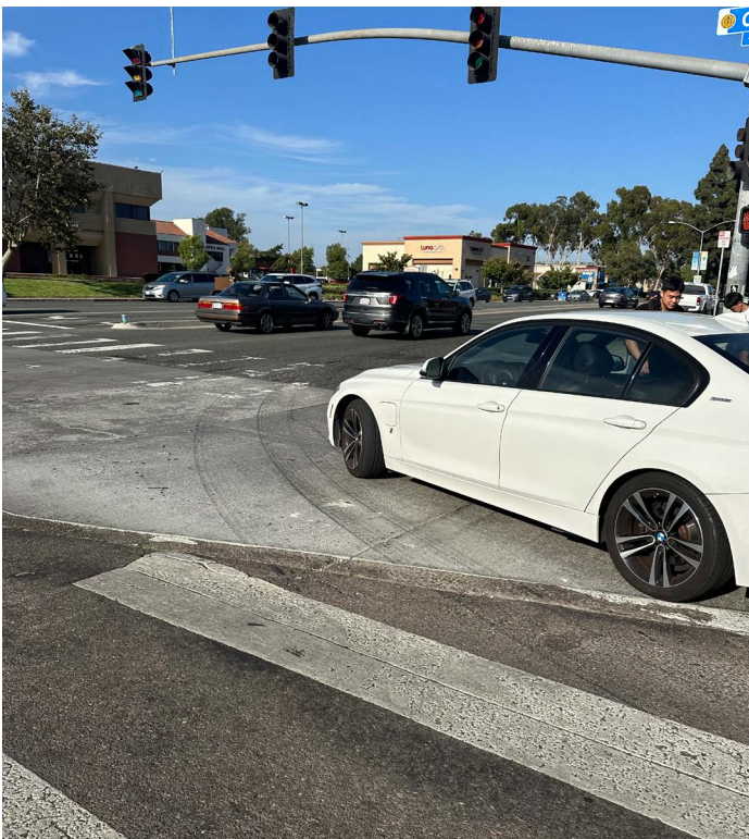
ABOVE: A driver on Camino Ruiz makes a high-speed right turn onto Mira Mesa Boulevard. On the pavement are tire marks, indicating that high turning speeds are common.
