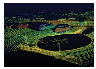
Figure 1: Example of LiDAR's perception of its surroundings (https://spectrum.ieee.org)
