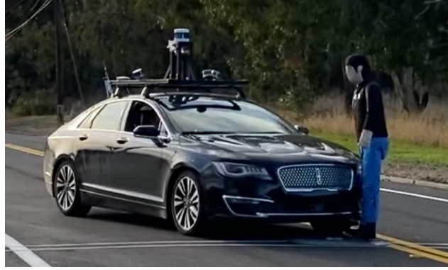
Figure 1: The Autonomous Vehicle (AV) and pedestrian dummy used for track testing. The picture shows the AV hitting the pedestrian during testing (test F1 Run 1, https://youtu.be/PehgLCGHF5U ), see Section 5 for details.
