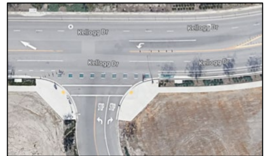
b) Lot Q and P driveway: dashed bike lane with green infill
