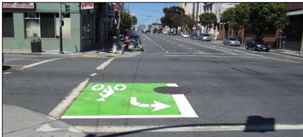
Figure 3-22: Two-Stage Bicycle Left Turn Box Example (11th & Howard Streets, SF)
