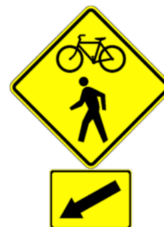
b) Trail crossing sign assembly (W11-15 sign at top)
