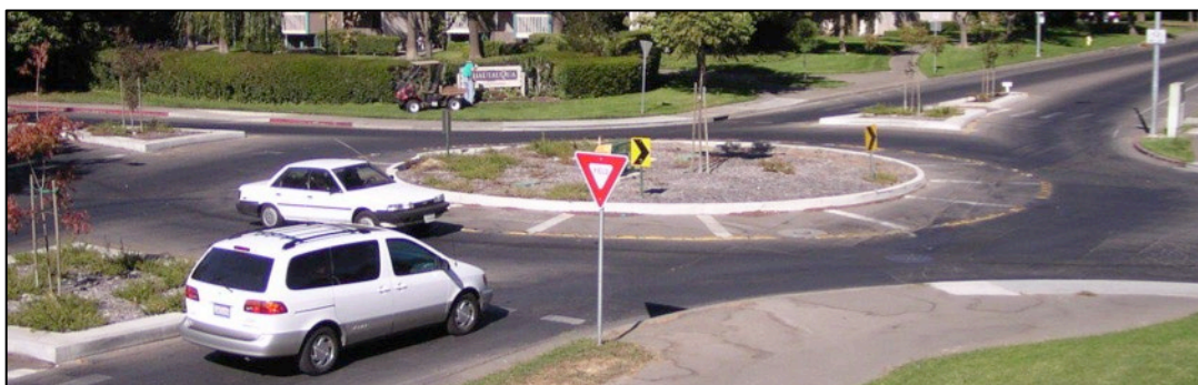
Figure 3-32: Truck Apron Using Radial Markers – Davis CA 2002 (Anderson & Alvarado)
