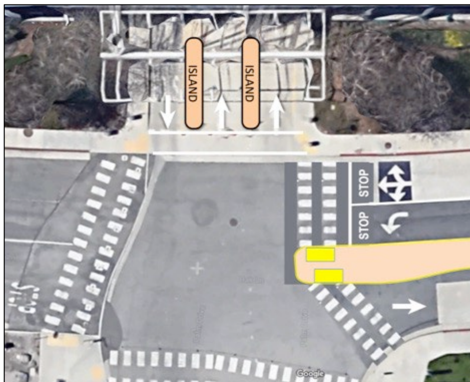
Figure 3-13: Concept For Enhancing East And North Crosswalks
