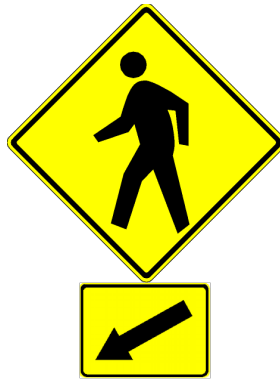
b) MUTCD standard warning sign assembly to be located at the crosswalk (note larger pedestrian symbol)
