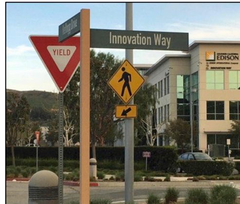
c) Street name signs distract from Yield and from warning signs (which is upstream of its crosswalk)
