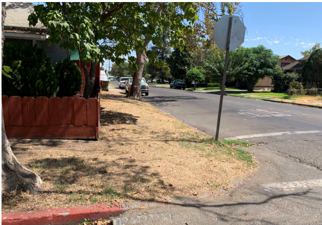
Top Left: Missing curb ramps on the southeast corner of High Street/Lane Street intersection.
