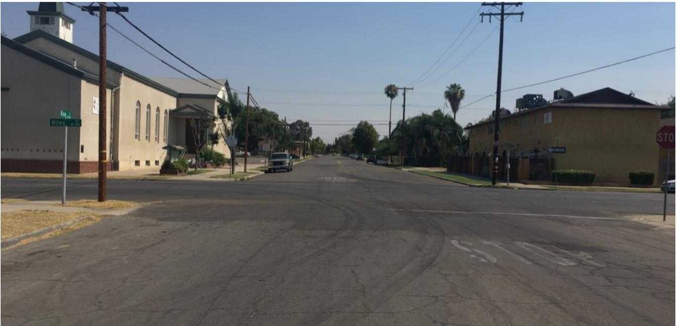
Faded stop sign and stop bar markings.
